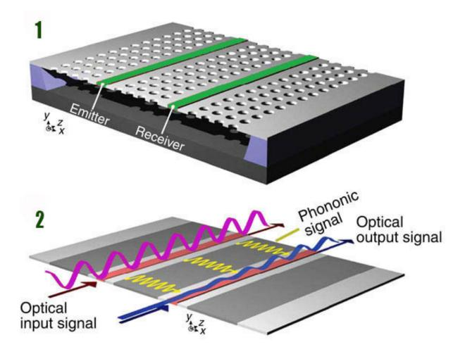
In the upper image, two green silicon optical waveguides are shown embedded in a gray photonic crystal membrane. In the bottom image, the violet and blue curves represent optical input and output signals; the yellow curves represent transduced phonon waves. Credit: Sandia National Laboratories
