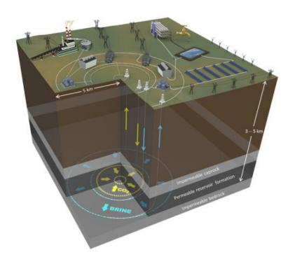
This integrated system would store carbon dioxide in an underground reservoir, with concentric rings of horizontal wells confining the pressurized CO2 beneath the caprock. Stored CO2 displaces brine that flows up wells to the surface where it is heated by thermal plants (e.g., solar farms) and reinjected into the reservoir to store thermal energy.
