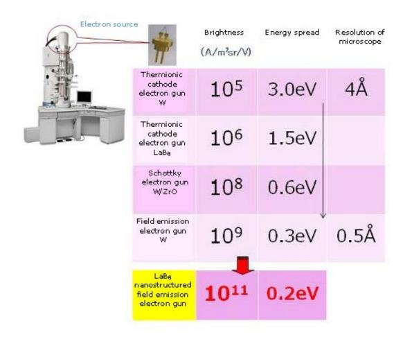
Comparison between the recently developed LaB6 nanowire field-emission electron source and the conventional electron source. The use of the new electron emitter allowed the development of the source of ultra-bright electron beams, with their energy spread being two-thirds of the energy spread associated with a contemporary electron emitter.
