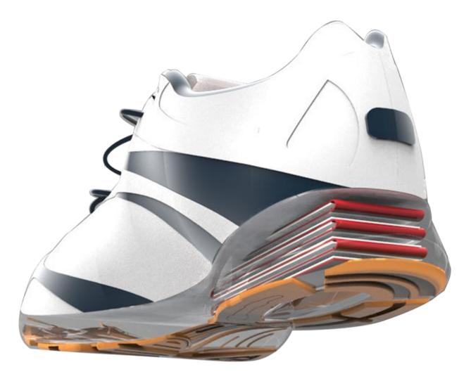
This is illustration shows how a triboelectric generator embedded in a shoe would produce electricity as a person walked. Credit: Zhong Lin Wang Laboratory
