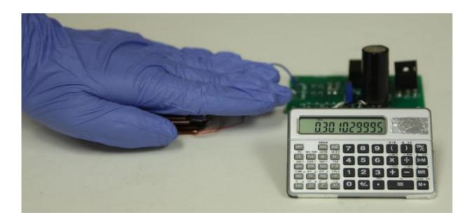
With this triboelectric nanogenerator and two-stage power management and storage system, finger tapping motion generates enough power to operate this scientific calculator. Credit: Credit: Zhong Lin Wang Laboratory
