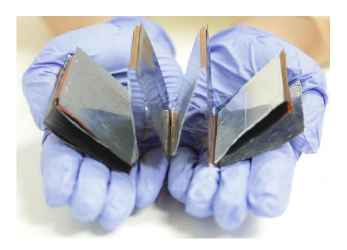
Triboelectric nanogenerators use a combination of the triboelectric effect and electrostatic induction to generate small amounts of electrical power from mechanical motions such as rotation, sliding or vibration. Credit: Zhong Lin Wang Laboratory
