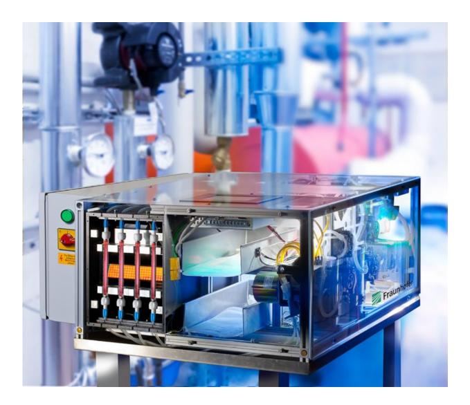
Online monitoring of water supply pipes: The biological broadband sensor AquaBioTox reacts immediately to toxic substances in water.
