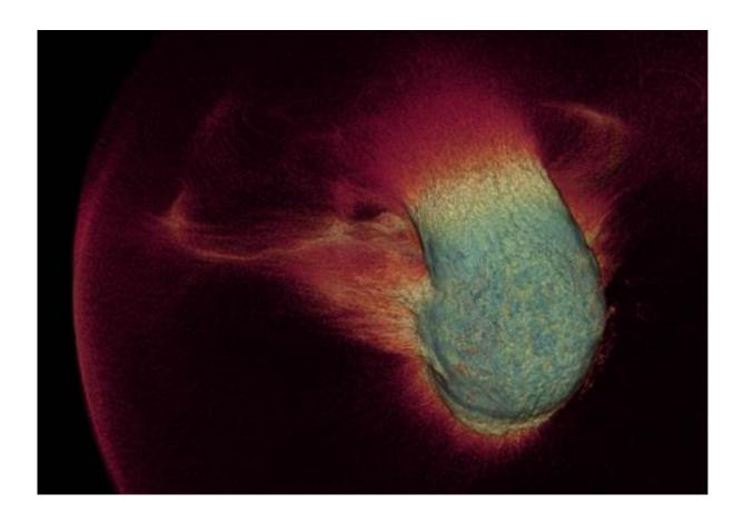
Proton density after laser impact on a spherical solid density target: irradiated by an ultra-short, high intensity laser (not in picture) the intense electro-magnetic field rips electrons apart from their ions and creates a plasma. By varying the target geometry and laser properties, scientists could find optimal regimes to accelerate high quality, directed ion beams that are currently studied in accompanying experiments. Credit: Axel Huebl, HZDR, David Pugmire, ORNL.
