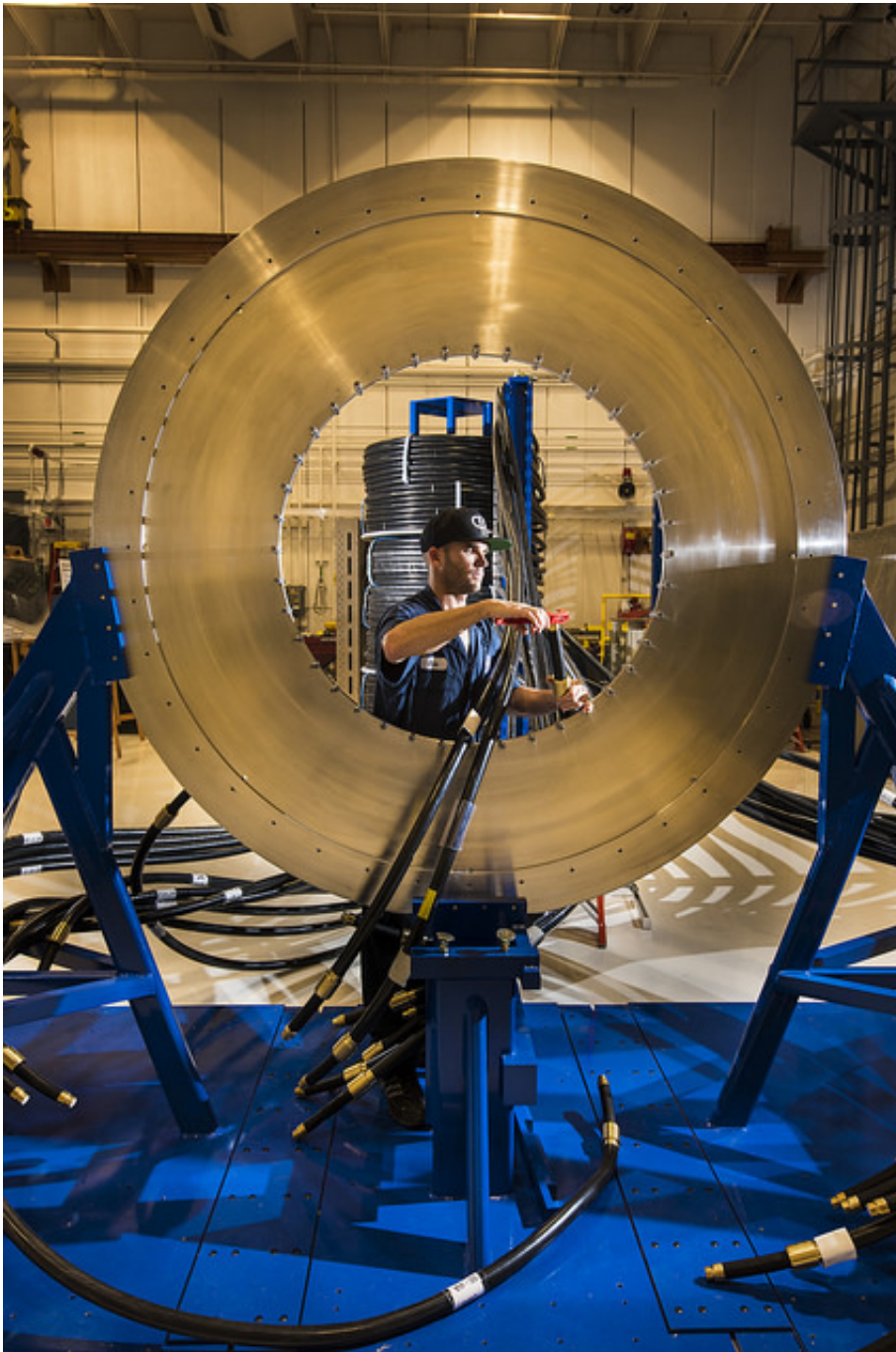
Sandia National Laboratories technician Eric Breden installs a transmission cable on the silver disk that is the new pulsed-power machine's central powerflow assembly. Credit: Randy Montoya
