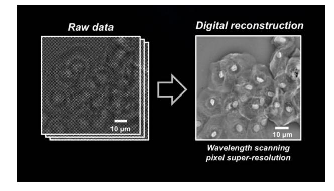
Raw data is transformed into the pixel super-resolution image. Credit: Ozcan Lab
