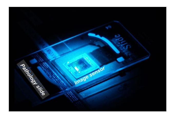
The image sensor of the wavelength scanning super-resolution apparatus collects a "stack" of images of the sample. Credit: Ozcan Lab
