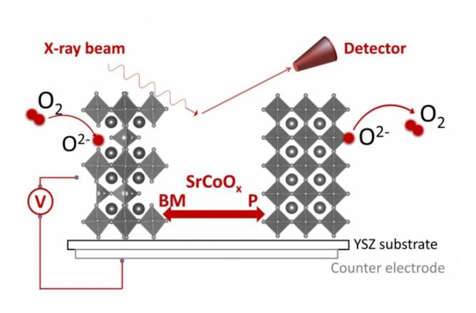
This diagram shows how an electrical voltage can be used to modify the oxygen concentration, and therefore the phase and structure, of strontium cobaltites. Pumping oxygen in and out transforms the material from the brownmillerite form (left) to the perovskite form (right).
