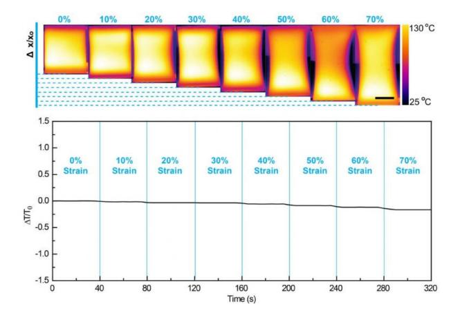
Infrared images of the heater show it being stretched to 70% longer than its original size with almost no decrease in the heater's temperature. Credit: Byeong Wan An, et al. ©2015 American Chemical Society
