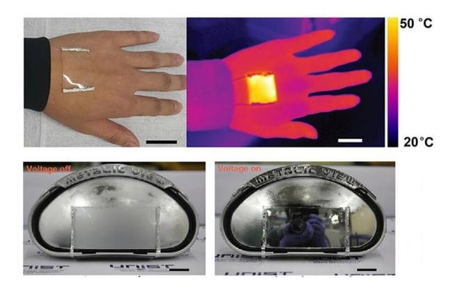
The stretchable, transparent heater could be used to warm the human body (where the black wrist strap can control temperature) or to defrost car mirrors. Credit: Byeong Wan An, et al. ©2015 American Chemical Society
