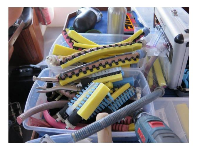
The team devised a modular design that allowed for easy in-field replacement and repairs -- and brought plenty of extra gripper components. Credit: Kevin Galloway, Wyss Institute at Harvard University
