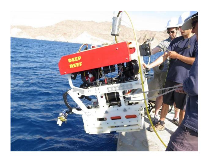
Soft robotic gripper is attached (lower left) to the remotely operated vehicle (ROV) as it is lowered into the Red Sea for a test dive. Credit: Kevin Galloway, Wyss Institute at Harvard University
