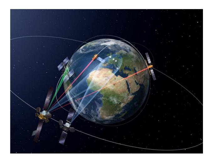
The European Data Relay System (EDRS) is designed to transmit data between low earth orbiting satellites and the EDRS payloads in geostationary orbit using innovative laser communication technology. Composed of a hosted payload (EDRS-A) on a commerical telecom satellite and a dedicated satellite (EDRS-C) in geostationary orbit, EDRS will dramatically increase the speed of data transmission for satellites in lower orbits and airborne platforms to relay their
