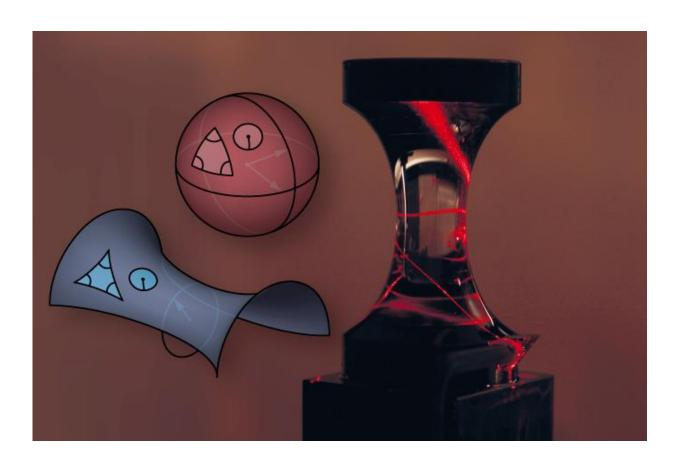
A laser beam in an experiment propagates along the two-dimensional surface of a glass object shaped like an hourglass, curling once around the middle of the object. This is an example of an object with negative surface curvature (like a saddle, for example), in contrast to an object with positive surface curvature, such as a sphere. Credit: Vincent Schultheiß
