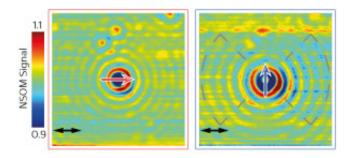
The electric and magnetic resonances of silicon nanoparticles are very different, and controlling them will enable the complex manipulation of light on the nanoscale. The color code indicates the intensity of the scattered light for electric- and magnetic resonances. Credit: Reprinted with permission from Ref 1. Copyright 2015, AIP Publishing LLC
