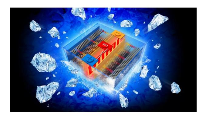
An all-climate battery that rapidly self-heats battery materials and electrochemical interfaces in cold environments. Credit: Chao-Yang Wang, Penn State
