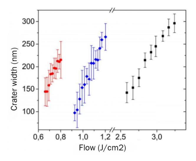
Fig. 3. The dependence of the width of the craters from the laser radiation power. Red - for microspheres of 2.25 microns in size, blue - 1.15 microns, black - without microspheres. Credit: ACS Publications/*Applied Materials & Interfaces*
