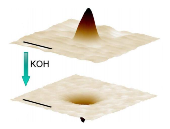
Fig. 2. The laser-treated surface of the glass before and after the application of alkali. (from the article)
