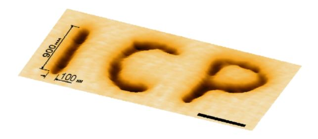
Fig. 5. ICP abbreviation applied to the glass. Credit: ACS Publications/Applied Materials & Interfaces
