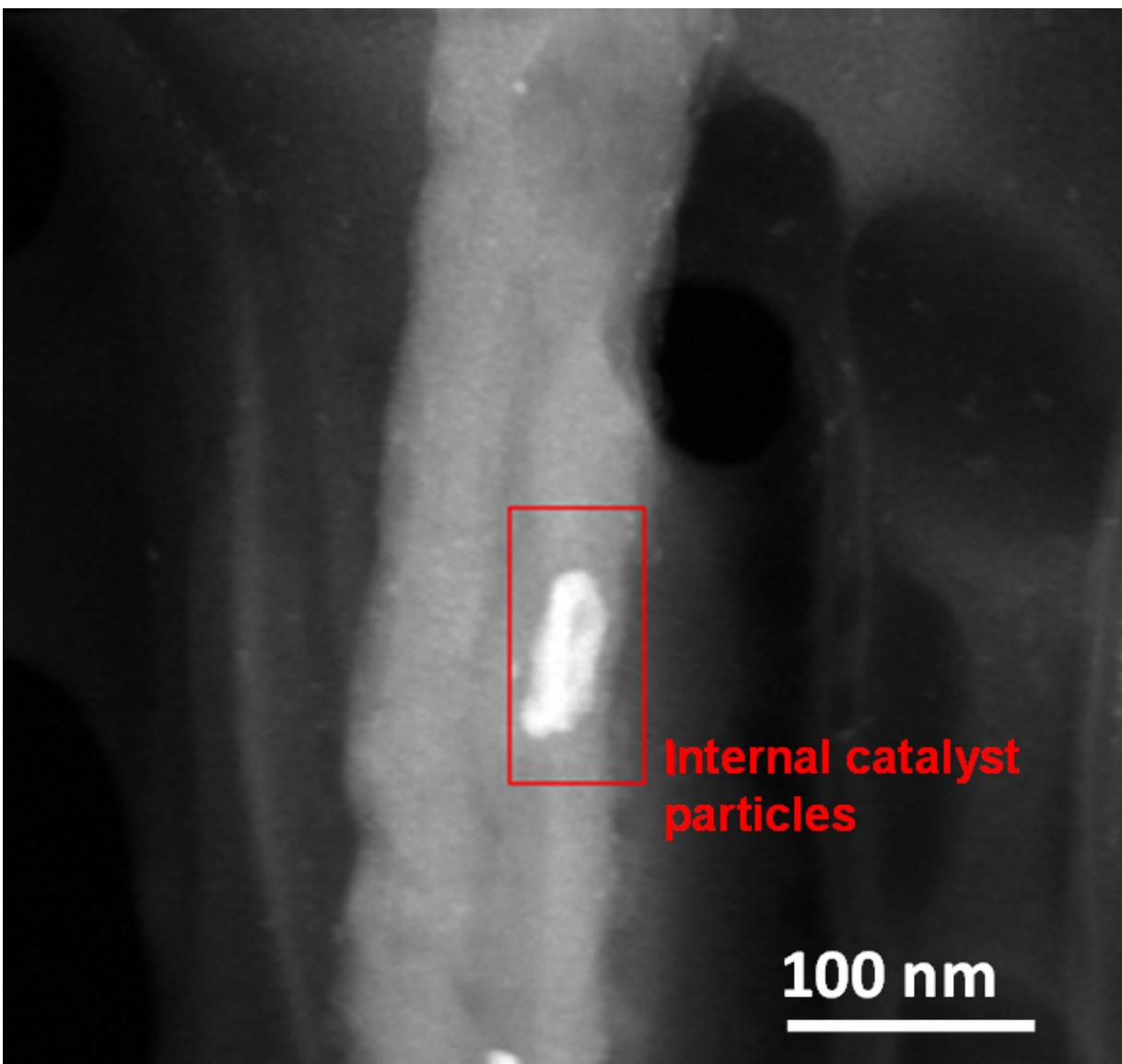
A multiwalled carbon nanotube cleaned with a process developed at Rice University and Swansea University shows iron catalyst residue has been removed from the surface, while most particles have been removed from inside the nanotube's walls. The process is expected to make nanotubes more suitable for applications like drug delivery and solar panels. Credit: Virginia Gómez Jiménez/Swansea University
