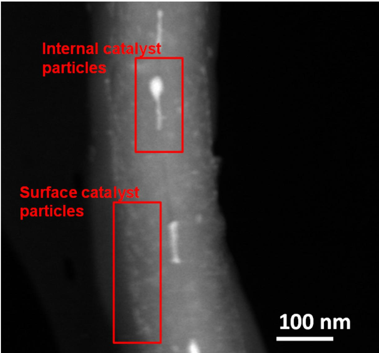
Multiwalled nanotubes before treatment with a Rice University/Swansea University process to remove catalyst residue from their surfaces and from inside. The process begins with heating the nanotubes in a standard kitchen microwave oven. Credit: Virginia Gómez Jiménez/Swansea University
