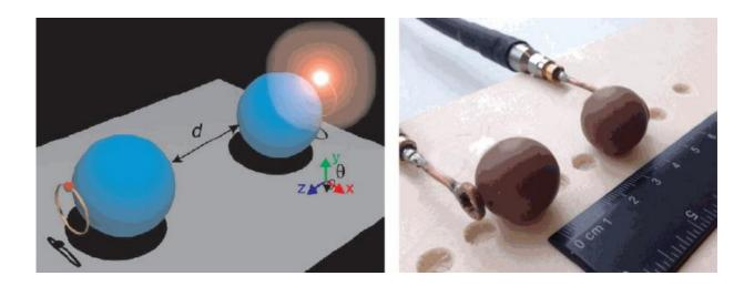
(Left) Illustration and (right) experimental setup of the wireless power transfer system. Power is transferred from one ceramic sphere to the other using the spheres' identical magnetic resonance. Credit: Song, et al. ©2016 AIP Publishing
