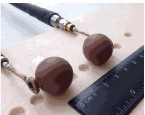
(Left) Illustration and (right) experimental setup of the wireless power transfer system. Power is transferred from one ceramic sphere to the other using the spheres' identical magnetic resonance. Credit: Song, et al. ©2016 AIP Publishing
