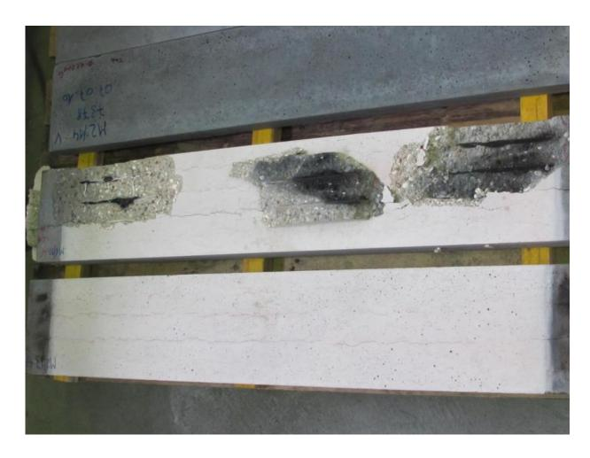
The SAP-containing concrete element resisted temperatures of about 1000 °C, and its capacitance was preserved. The slab made of concrete without SAP showed some severe spalling which reduced the loading capacity of the slab and raised the risk of a collapse.
