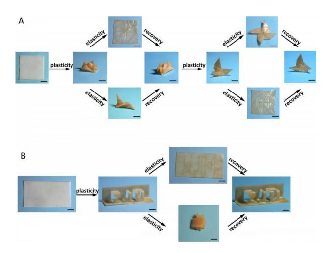
Shape manipulation via thermally distinct elasticity and plasticity. (A) Smart origami structures. (B) Smart kirigami structure. Credit: Dr. Qian Zhao and Dr. Tao Xie
