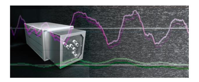
Japanese researchers have come up with a way to measure heartbeats remotely, in real time, and under controlled conditions with as much accuracy as electrocardiographs. The technology utilizes spread-spectrum radar to catch signals from the body and an algorithm that distinguishes heartbeats from other signals. Credit: Kyoto University
