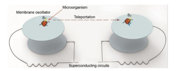
Quantum teleportation between two microorganisms is shown. The internal state (an electron spin) or the center-of-mass motion state of a microorganism on an electromechanical oscillator can be teleported to a remote microorganism on another electromechanical oscillator assisted with superconducting circuits. Credit: ©Science China Press
