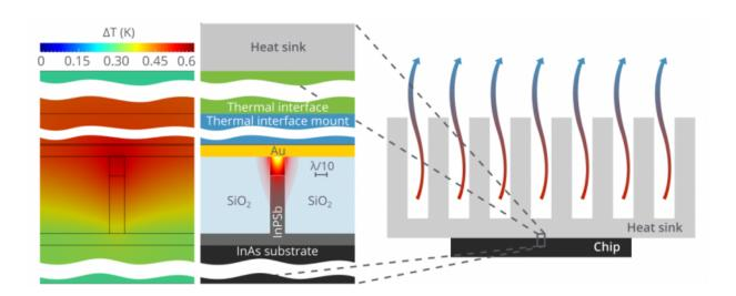
Temperature distribution in an active plasmonic waveguide on an optoelectronic chip with a cooling system
