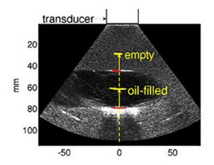
This ultrasound image shows a cavity filled with olive oil. Dashed and solid vertical lines indicate the proton beam path through material with relative stopping powers near 0 and 1, respectively. Bragg peaks from both empty and filled cavities are overlaid in yellow. Overlaid in red are estimates of entrance point of beam into the material with high stopping power, in agreement with the ultrasound image.
