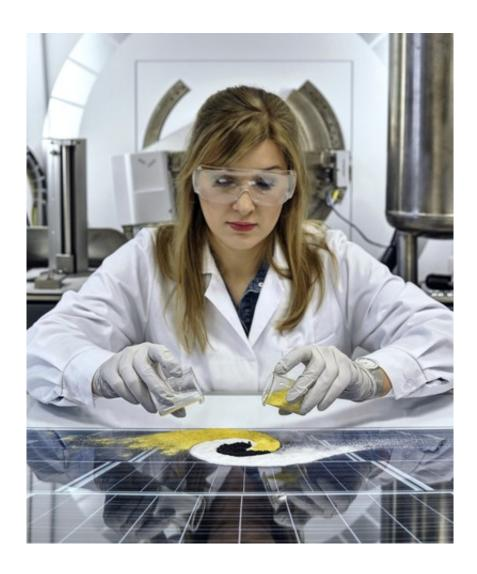
A simple, fast and safe method of obtaining perovskites has been discovered by scientists from IPC PAS in Warsaw, Poland. The perovskite (a black powder) is milled from two powders: a white one, methylammonium iodide, and a yellow one, lead iodide. Credit: IPC PAS, Grzegorz Krzyzewski
