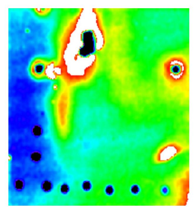
ORNL's Ralph Dinwiddie uses infrared cameras to create heat maps of working materials that reveal their thermal properties and subsurface structure. This 1998 image of an aging aircraft's engine cowling revealed severe subsurface corrosion. Credit: Oak Ridge National Laboratory, U.S. Dept. of Energy; Ralph Dinwiddie
