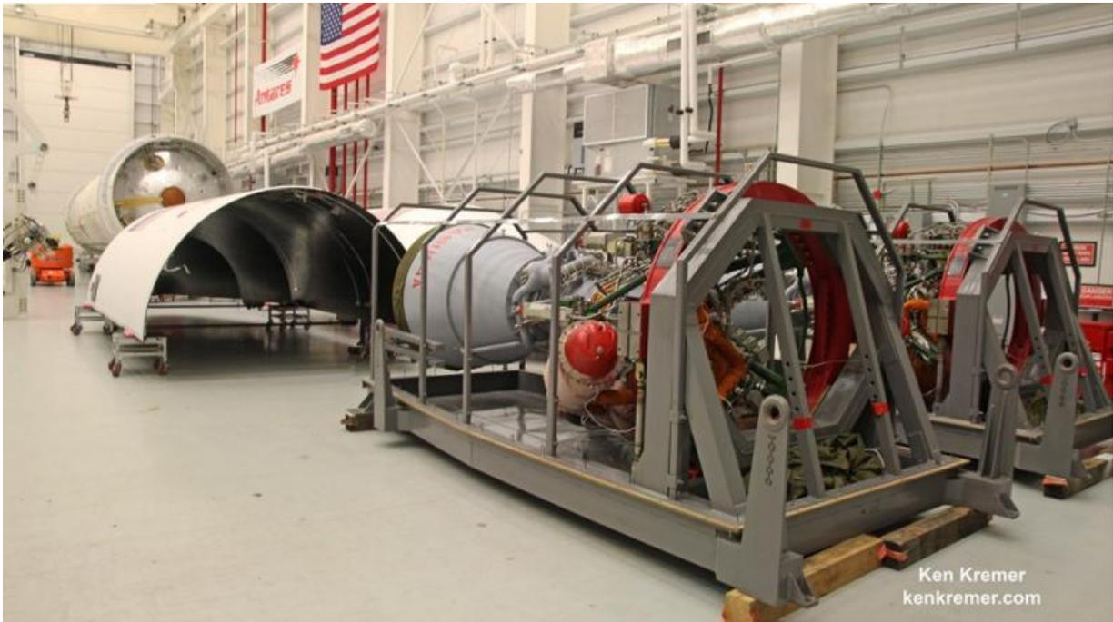
All major components of Antares are in place and undergoing launch vehicle integration at Orbital ATK's Horizontal Integration Facility at NASA's Wallops Flight Facility. Credit: Ken Kremer/kenkremer.com
