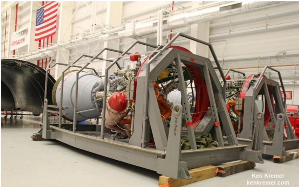
Up close view of two new RD-181 engines that will power the revamped Orbital ATK Antares rocket to orbit. Credit: Ken Kremer/kenkremer.com
