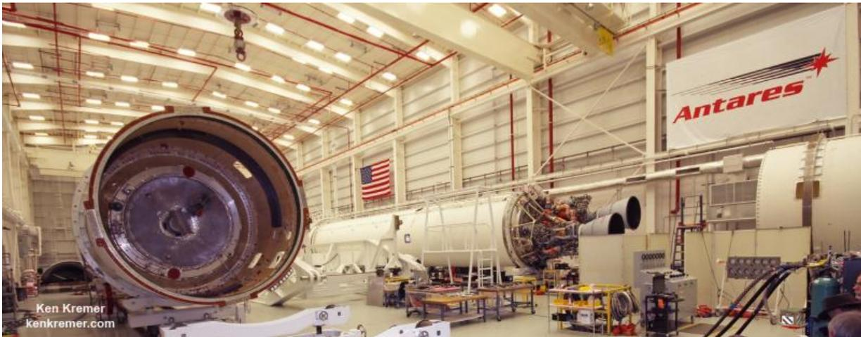
The new RD-181 engines are installed on the Orbital ATK Antares first stage core ready to support a full power hot fire test at the NASA Wallops Island launch pad in March 2016. Credit: Ken Kremer/kenkremer.com
