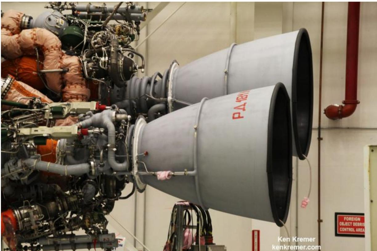
The new RD-181 engines are installed on the Orbital ATK Antares first stage core ready to support a full power hot fire test at the NASA Wallops Island launch pad in March 2016. New thrust adapter structures, actuators, and propellant feed lines are incorporated between the engines and core stage.
