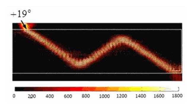
A self-collimated one-way light beam can be steered inside a photonic crystal using gradient magnetic fields. Credit: Li, et al. ©2015 AIP Publishing
