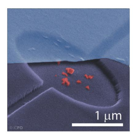
False colour scanning electronic micrograph (SEM) of hybrid graphene-NV near-field nano-optomechanical system. Credit: ICFO
