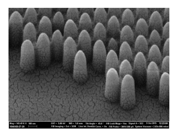
A scanning electron miscroscope photograph shows the pyramid-like nanostructures engraved onto glass: at 200nm they are 100 times smaller than a human hair. Controlling the surface morphology at the nanoscale allows scientists to tailor how the glass interacts with liquids and light with high precision.
