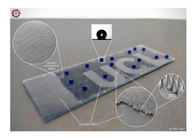
A smart glass prototype developed by the UCL team. The dark areas are decorated with the nanostructures, which significantly suppress reflections. They also repel water forcing it to form nearly spherical droplets and preventing it from wetting the surface of the glass. The UCL logo is made of untreated glass and appears significantly more reflective compared with its surrounding region.
