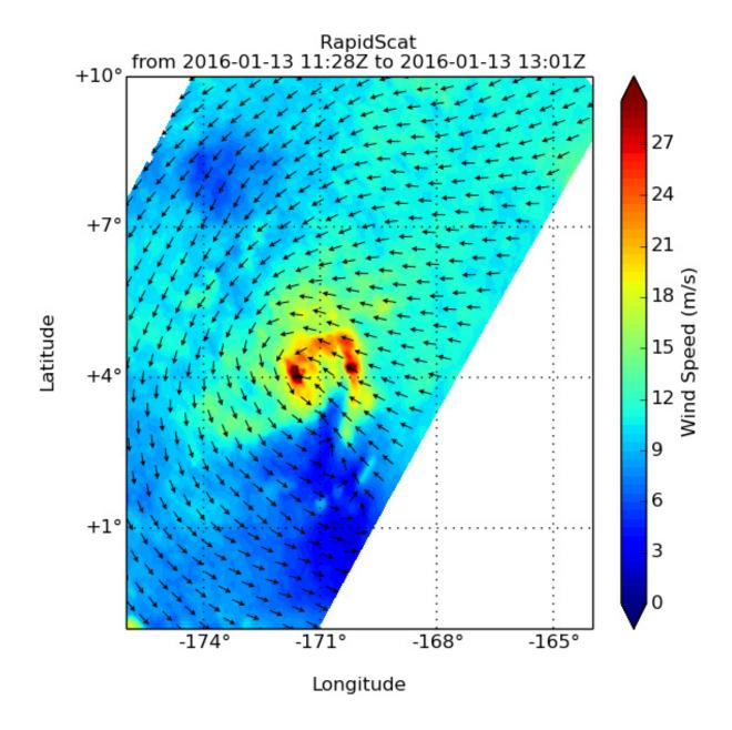
On Jan. 13 at 1200 UTC (7 a.m. EST), NASA's RapidScat instrument measured strongest sustained winds near 27 meters per second (60.4 mph/97.2 kph) both east and west of center. Credit: NASA JPL, Doug Tyler
