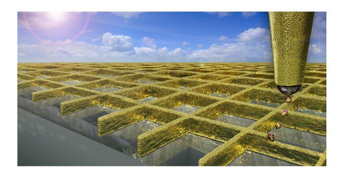
With a special mode of electrohydrodynamic ink-jet printing scientists can create a grid of ultra fine gold walls. Credit: Ben Newton / Digit Works
