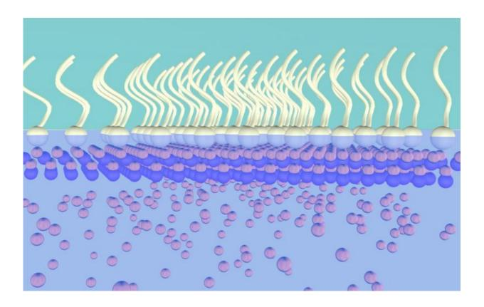
The new nanoscale manufacturing process draws zinc to the surface of a liquid, where it forms sheets just a few atoms thick. Credit: Xudong Wang
