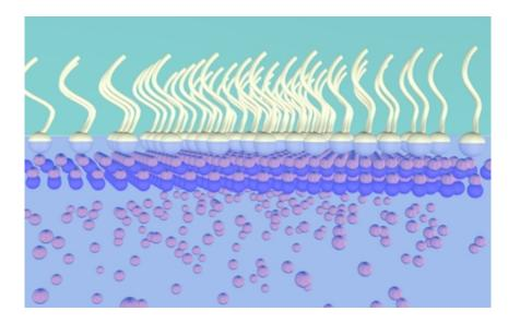
Schematic illustration of the formation of ZnO nanosheets directed by surfactant monolayer
