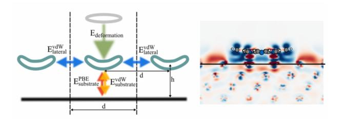
Schematic depiction of different energy terms contributing to the adsorption energy, and charge density difference of 2H-P after adsorption onto Cu(111) at 12.8 Angstrom separation. Credit: M. Müller/TU Munich
