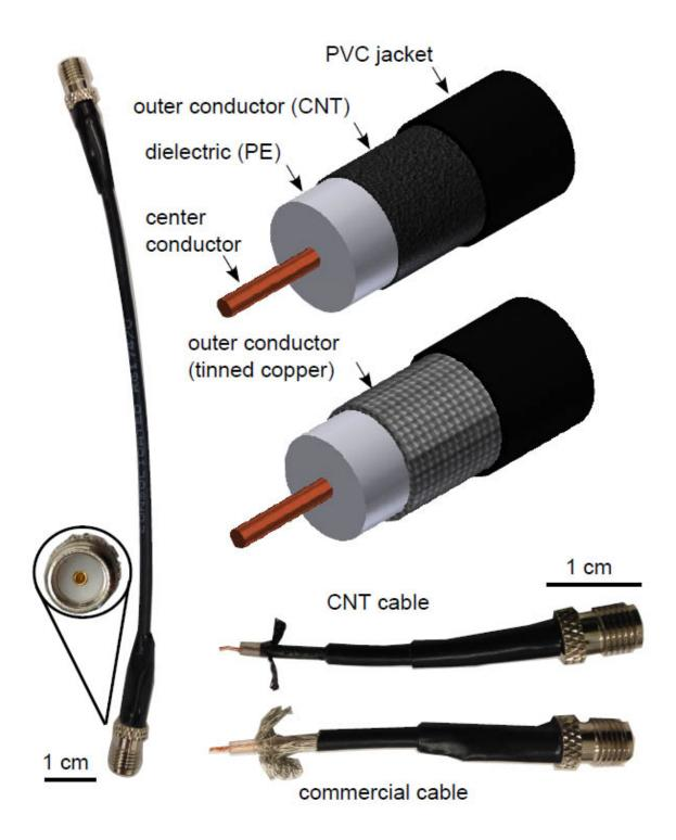
Replacing the braided outer conductor in coaxial data cables with a coat of conductive carbon nanotubes saves significant weight, according to Rice University researchers. Credit: Pasquali Lab/Rice University
