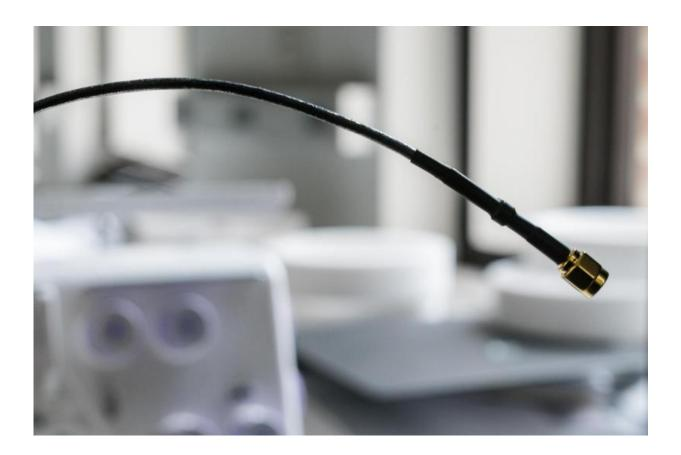
A coating of carbon nanotubes, seen through a clear jacket, replaces a braided metal outer conductor in an otherwise standard coaxial data cable. Rice University scientists designed the cable to save weight for aerospace applications. Credit: Jeff Fitlow/Rice University
