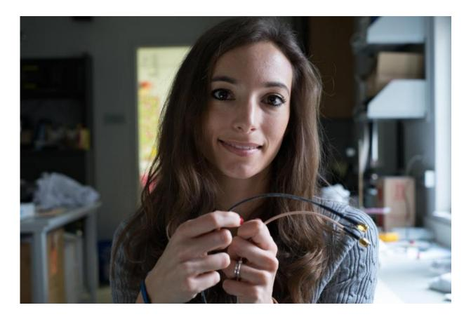
Rice University research scientist Francesca Mirri holds a standard coaxial data cable (bottom) and a new cable with an outer conductor of carbon nanotubes. Replacing the braided metal outer conductor with a conductive nanotube coating makes the cable 50 percent lighter, Mirri said. Credit: Jeff Fitlow/Rice University
