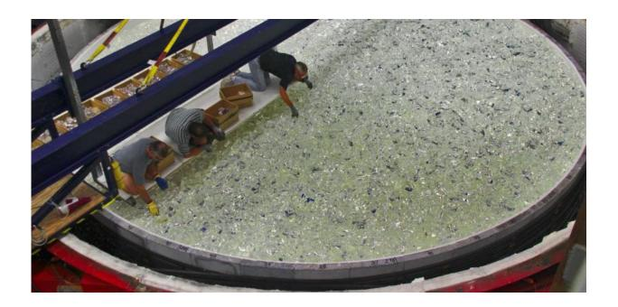
20 tons of Ohara E6 borosilicate glass being loaded onto the mold of one of the GMT's mirrors. Credit: Ray Bertram, Steward Observatory, CC BY-ND
