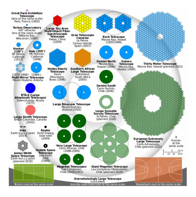
Size comparison of optical telescopes' primary mirrors. Credit: Cmglee, CC BY-SA
