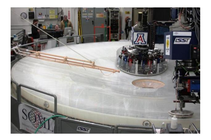
An 8.4-meter mirror for the Large Synoptic Survey Telescope being polished at the Richard F. Caris Mirror Lab. Credit: Steward Observatory, CC BY-ND
