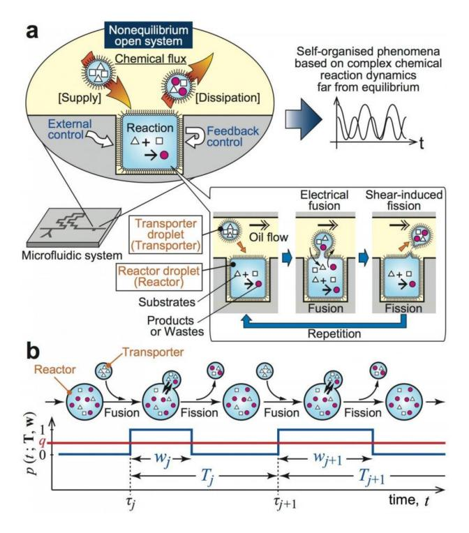
Schematic diagram of chemical reactions far from equilibrium in a droplet openreactor system controlled by pulse-density modulation. (a) In the droplet openreactor system, the supply of substrates and the dissipation of products/wastes into/out of the reaction system are sustained, inducing self-organized phenomena based on complex chemical reaction dynamics far from equilibrium. The
