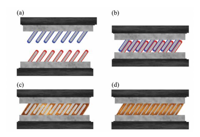
a) Coated rods are arranged along a substrate, like angled teeth on a comb. b) The teeth are then interlaced. c) When indium and galium come into contact, they form a liquid. d) The metal core of the rods turns that liquid into a solid. The resulting glue provides the strength and thermal/electrical conductance of a metal bond. From "Advanced Materials & Processes," January 2016
