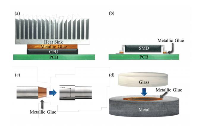
A schematic illustrating applications of metallic glue: a) A CPU on a printed circuit board connected to a heat sink. b) A surface mount device being attached to a printed circuit board. c) A press-fit pipe fitting for environments where welding is dangerous or impossible. d) A glass plate being attached to metal with a different thermal-expansion coefficient to cover a cavity with a hermetic seal. From "Advanced Materials & Processes," January 2016
