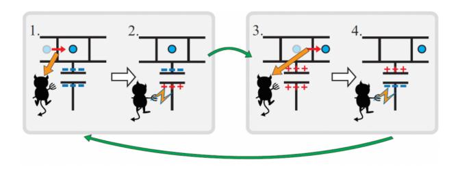
An autonomous Maxwell's demon. When the demon sees the electron enter the island (1.), it traps the electron with a positive charge (2.). When the electron leaves the island (3.), the demon switches back a negative charge (4.). Credit: Jonne Koski
