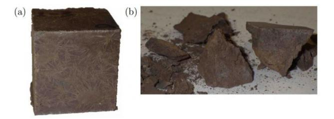
Cube specimen (a) before and (b) after unconfined compression test. Credit: arXiv:1512.05461 [cond-mat.mtrl-sci]
