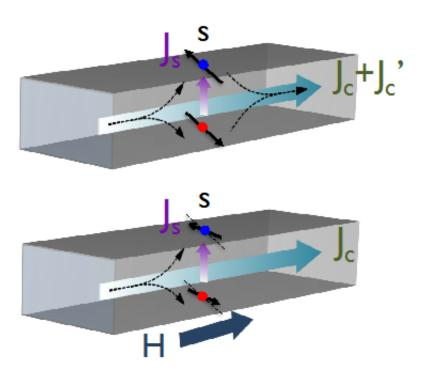
Top: Schematic of the direct spin Hall effect (and its inverse) in a thin film of a material with strong spin-orbit coupling. Bottom: schematic of the Hanle magnetoresistance effect when an external magnetic field is applied. Credit: PRL
