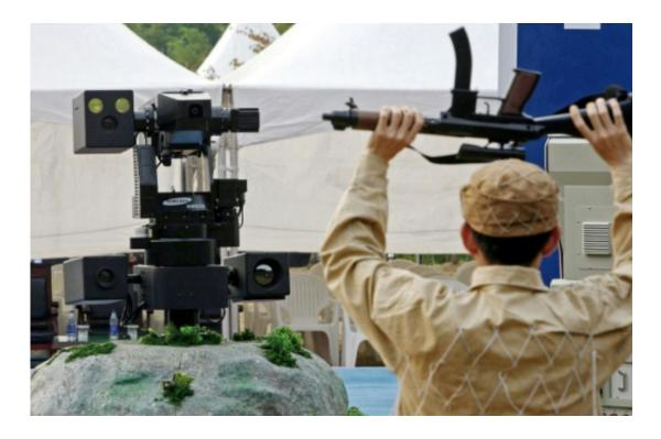
A sentry robot freezes a hypothetical intruder by pointing its machine gun during a 2006 test in Cheonan, South Korea
