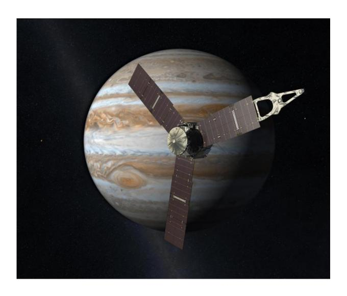
Launching from Earth in 2011, the Juno spacecraft will arrive at Jupiter in 2016 to study the giant planet from an elliptical, polar orbit. Juno will repeatedly dive between the planet and its intense belts of charged particle radiation, coming only 5,000 kilometers (about 3,000 miles) from the cloud tops at closest
