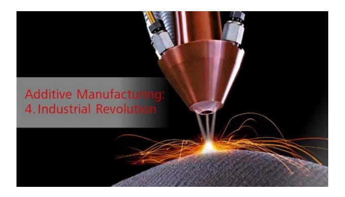
D printing with metal powder and a laser: laser direct metal deposition (LMD) involves melting metal particles in the focus area of a laser beam. A workpiece made from solid metal is produced, made purely from CAD data without a die casting mold and milling machines. Credit: Trumpf GmbH + Co. KG
