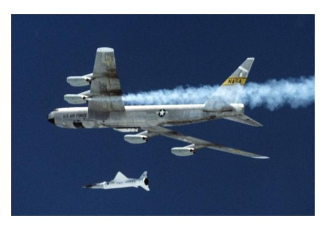
X-43 rocket plane dropped from a B-52, seconds before igniting its scramjet engines and reaching a world record-holding 10,000km/h (Mach 9.8). Credit: NASA
