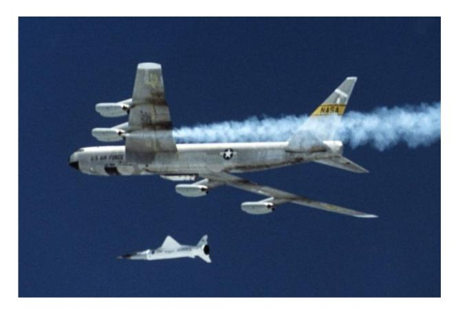
X-43 rocket plane dropped from a B-52, seconds before igniting its scramjet engines and reaching a world record-holding 10,000km/h (Mach 9.8). Credit: NASA
