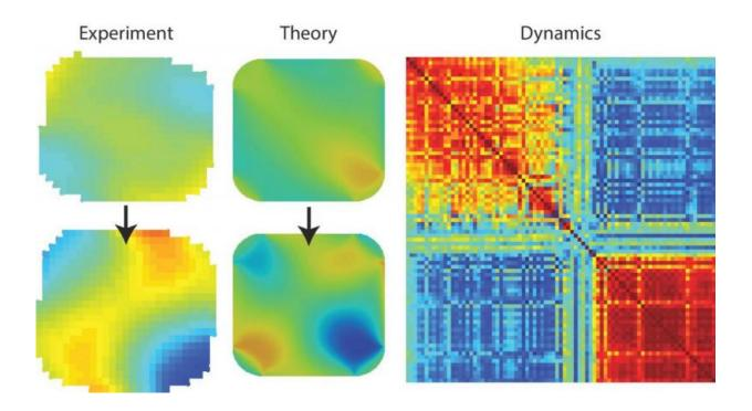
Comparison between experimental and calculated strain distributions in the hydrogen-poor phase. The strains are consistent with a trapped hydrogen-rich surface layer. Middle: Comparison between experimental and calculated strain distributions in the hydrogen-rich phase. The strains are dominated by elastic effects. Right: The time correlations in the displacement field that show evidence of aging and avalanching during the phase transformation.
