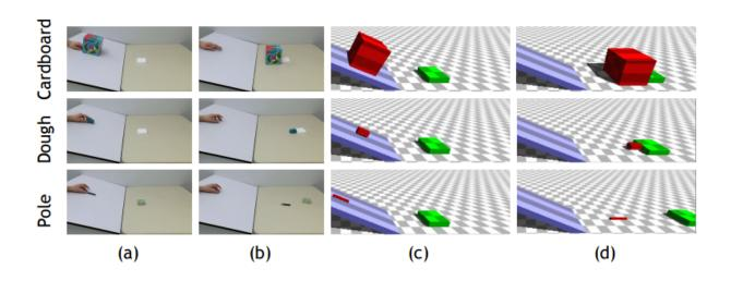
Researchers fed their physics prediction system videos of collisions, shown as screenshots in (a) and (b), which were then converted into simulations generated by the 3-D physics engine, shown in (c) and (d).
