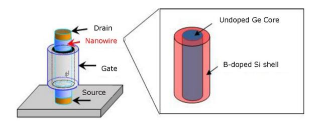
Schematic of a vertical transistor and an expanded view of its core-shell nanowire part.
