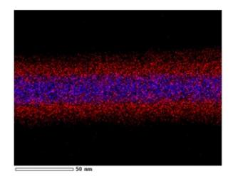
An EDX (energy-dispersive X-ray spectroscopy) image of a Ge/Si core-shell nanowire created by a CVD process. (Red, Si area; blue, Ge area.)
