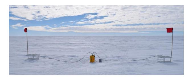
Phase sensitive radar system used by the Scripps Oceanography team to collect data. Credit: Scripps Oceanography/Oliver Marsh
